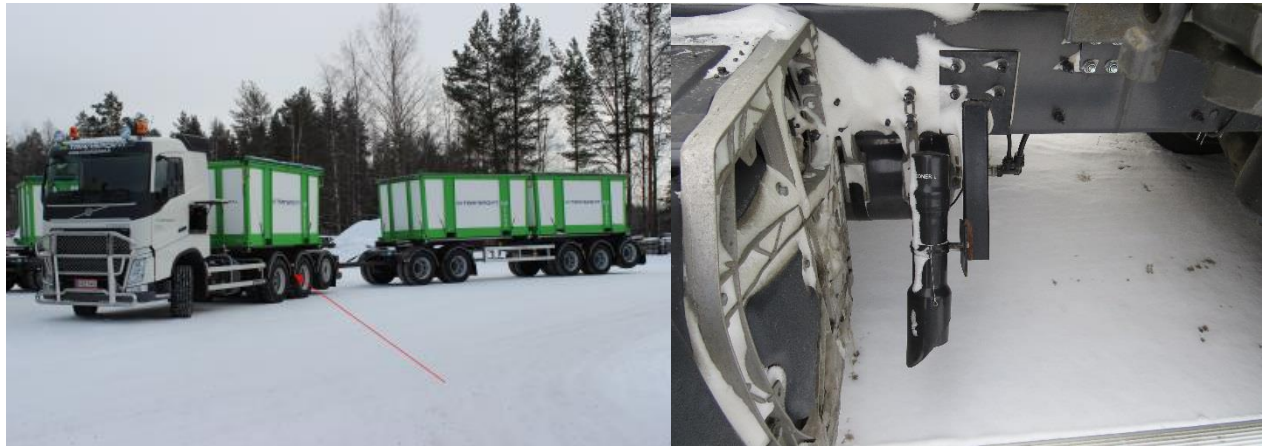
Figure 3. Left image: a heavy Transpoint ore transport combination truck. Right image: the externally visible road surface observation equipment installed onto the truck. The location of the equipment on the truck is indicated by a red arrow on the left image.
